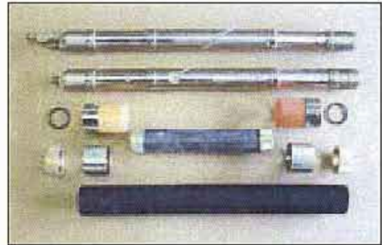
Pressuremeter probe with its components
